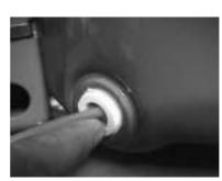
8- Push lock ring in the PTC block (until contact with PTC)
